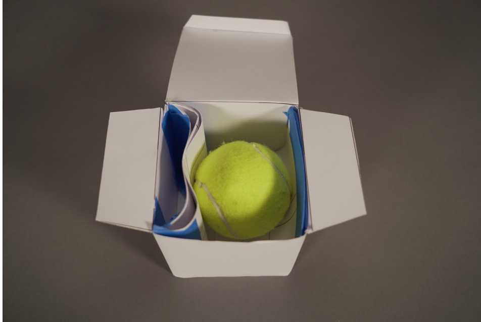
Example 2- Inserts attached to the box from the insides Each side layers cardstock in different directions to let the ball give into the insert.
