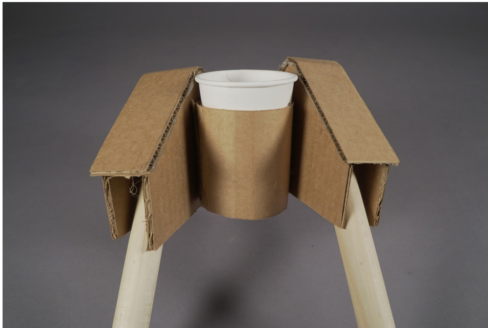
Example adaptation for the dowels to pick up the disposable coffee cup and tilt the beverage into a mouth, and then set it back down.
